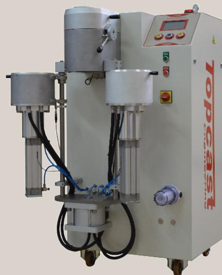
In order to increase the productivity, the system has been conceived with 2 loading chambers and one melting chamber. This configuration allows for melting the next ingot while the previous one is cooling. This overlapped working mode is also important to decrease the running cost of the process because they are mainly related to the graphite mould consumption. A colder graphite mould in output increases the life of the same.
