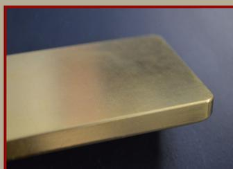
The TIP furnaces are designed to manufacture any size of ingots, from 100 g to kilo-bar either in gold or silver. The ingots are obtained by melting the pre-weighted grains in a graphite mould placed inside the vacuum chamber and then by cooling appropriately the ingot during the solidification phase.
