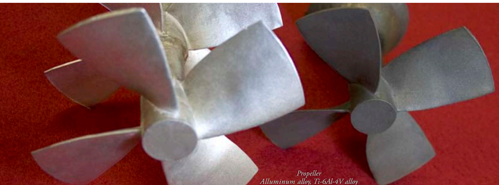
Compressor impeller ZL-105, ZL201 alloy, Ti-6Al-4V alloy
